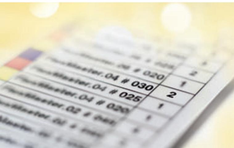
*You will receive our Torque CARDS with each of the endodontic handpieces. The recommended torque step for each individual file in your selected file system is specified on these cards.*
