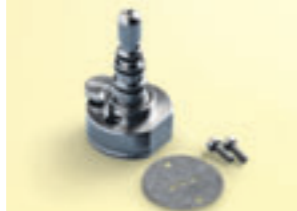
REF 6051911 Adapter for Morita turbines (PAR-DI) To attach: snap the turbine into the adapter. To detach: Press the small button on the adapter and detach the instrument.
