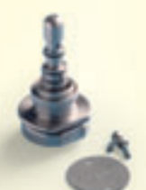
REF 6085745 OSADA OFJ-MZL To attach: Snap the turbine into the adapter. To detach: Press the bottom plate on the adapter and detach the turbine.
