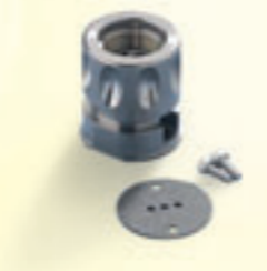
REF 6051846 Midwest adapter for quick connect (4, 5, 6 holes) To load: Align the instrument to fit the holes and press down. To unload: Press the ring and pull off the instrument.
