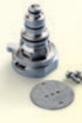
REF 6051887 Star swivel adapter To load: Turn the basic plate of the adapter to the right and click the turbine onto the adapter. To unload: Turn the basic plate of the adapter to the right and pull the turbine off the adapter.
