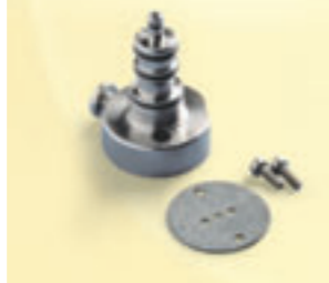
REF 6051713 Bien Air turbine adapter To load: Click the turbine onto the adapter. To unload: Push the small button on the adapter and remove the instrument.
